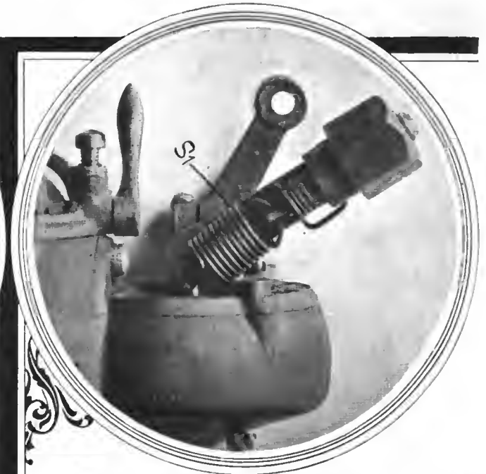
Fig. 3—Adjustment of auxiliary air mechanism in the position of fast running, requiring the maximum volume of air
